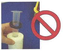
This shows the INCORRECT way to re-install your carbon filter assembly. This will prevent the necessary watertight seal, allowing the untreated water to bypass the carbon filter and UV process, rendering the water undrinkable.
