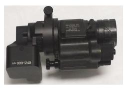
The OnX2 is the most innovative way to capture night vision images through the night vison lens, in real time. The video is a perfect image of what the night vision device is seeing. Following this example, the OnX3 is the thermal equivalent.
