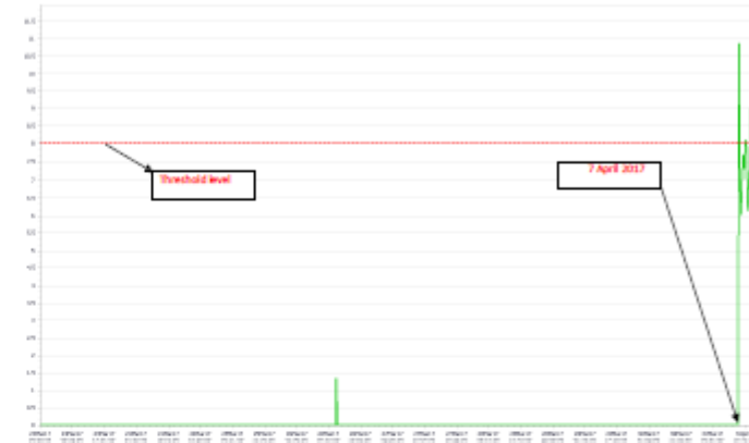
Figure 11: Unbalance / misalignment / coupling / bearing parameter of equipment TA 2000 COMPRESSOR
