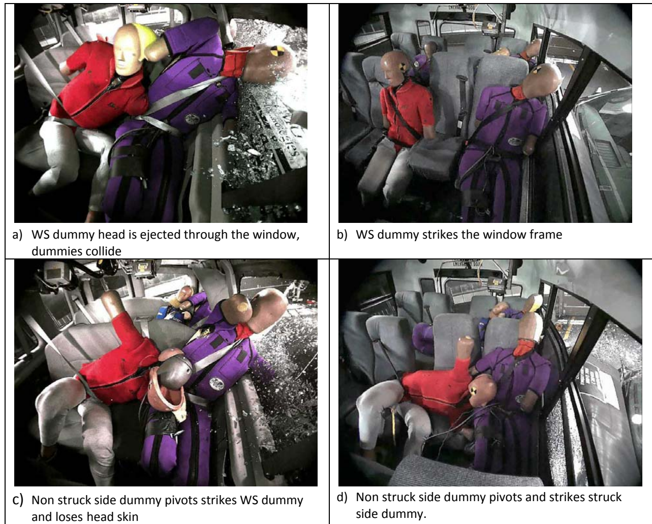
Figure 14. Motion during the crash of the second row occupants seated in the E350 (left) and MFAB (right)
