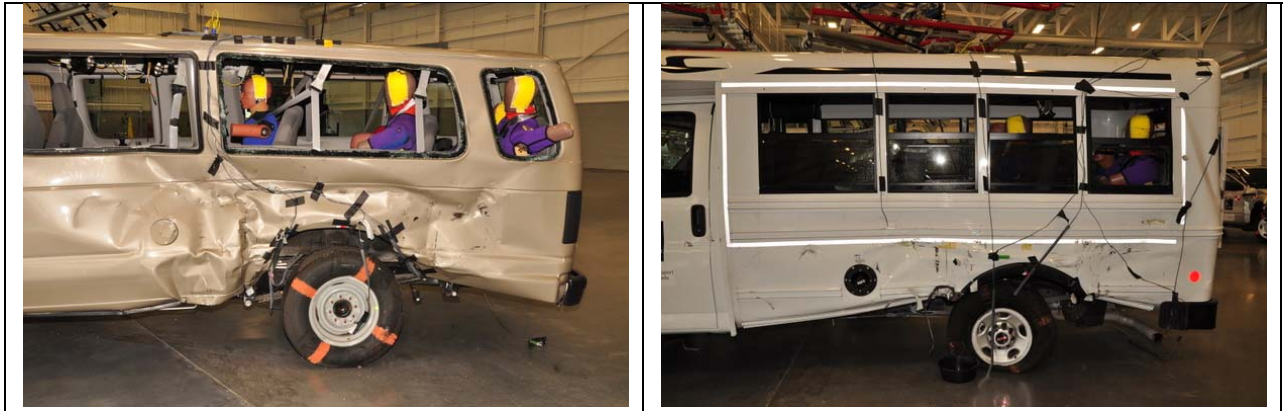
Figure 8. Location of impact point and view of imprint left by the F150 on the E350 (left) and MFAB (right).
