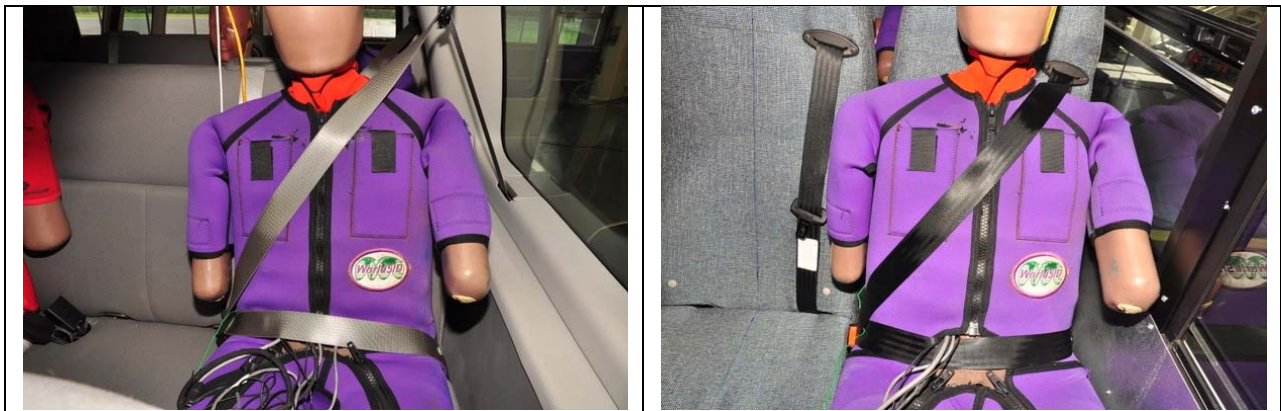
Figure 12. Comparison of interior trim and seatbelt anchorages in the E350 (left) and MFAB (right).
