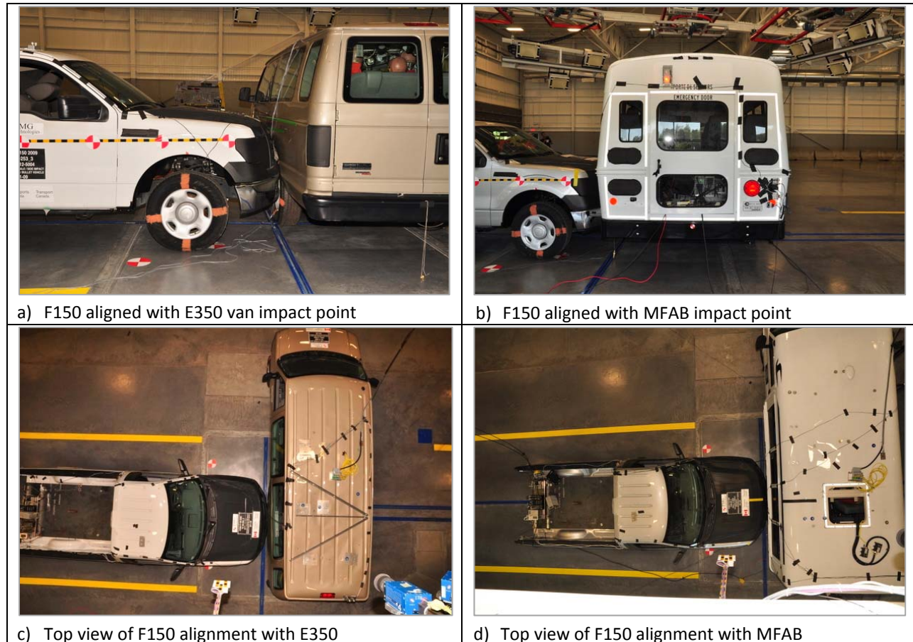
Figure 1. Test configuration for the paired comparison side impact test.
