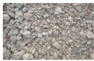
**21AA Slag** stone is larger particles use as a sub base for pavers. This stone is used under slag stone for a better more sturdy base. 1ton covers 40sq. ft. 4-5ö base.
