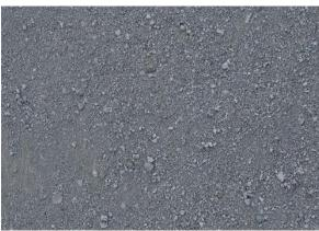
**30A Slag** sand is blue/grey in color. It is used as a top layer base under pavers and wall stone. 1 ton covers 40-50 sq. ft. 4-5ö base.
