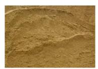
**Pool/Mason sand** is tan in color. A clean non packing sand used in sand boxes and under pools.
