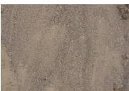
**2NS sand or sharp sand** is a coarse sand used under pavers and cement. It can be compacted.
