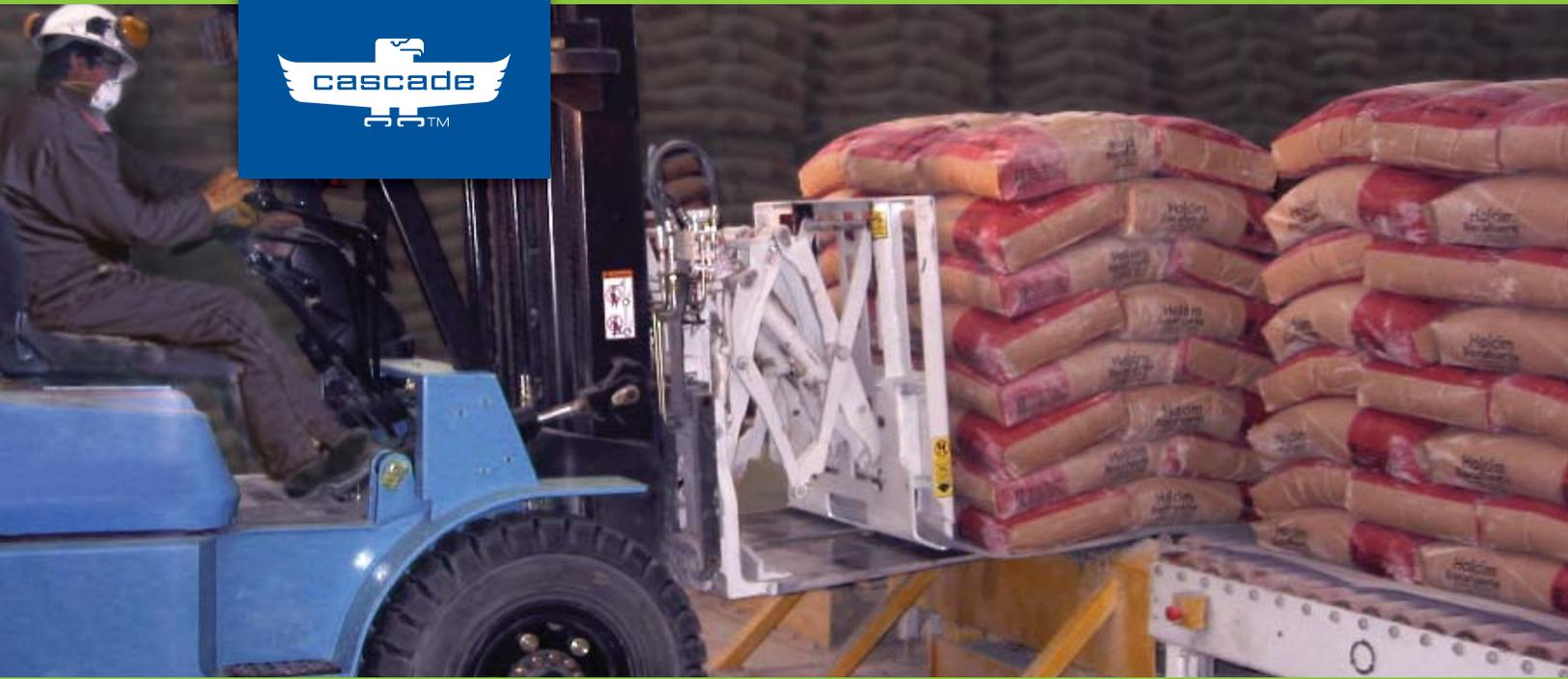
Pallet-Free Cement Handling with Heavy Duty Push/Pulls from Cascade.
