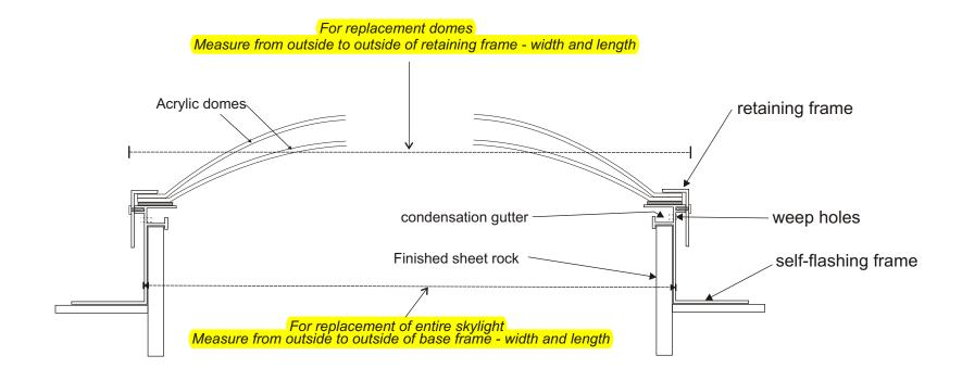
Self-Flashing Detail - Typical
