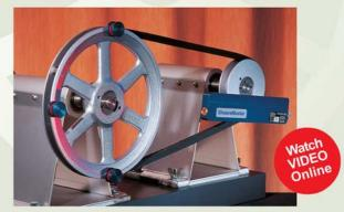
Measuring pulley misalignment with a straightedge or string is cumbersome and requires two people. One person does it easily with **SHEAVEMASTER**<sup>®</sup>!
